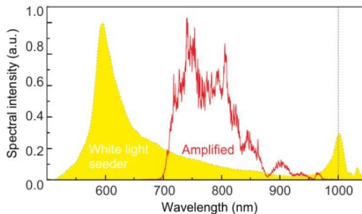
Figure 4: The spectral profile of the WLG output and the amplified output from the OPA stage.
