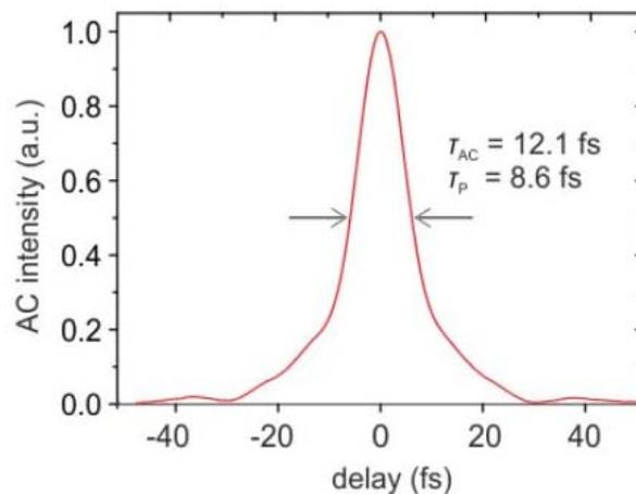
Figure 5: Autocorrelator measurements show that the White Dwarf output pulse width is 8.6 fs.
