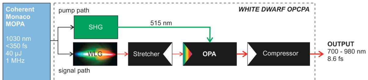
Figure 3: The Main components of the White Dwarf.
