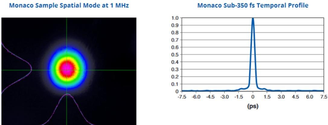
Figure 2: The Monaco is a Yb-fiber MOPA with a circular TEM00 output beam and a pulse width < 350 fs.
