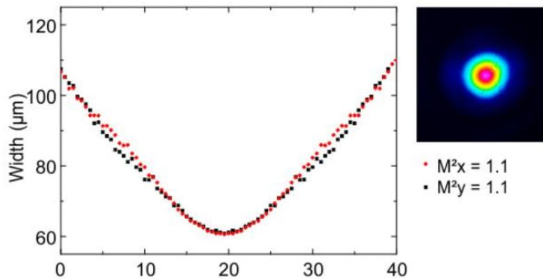
Figure 7: The output is characterized by M2 values < 1.2 in both axes.
