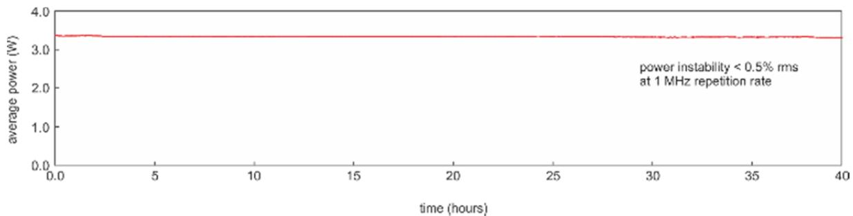
Figure 6: Long term power stability of the White Dwarf operating at a pulse width of 8.6 fs and a 1 MHz repetition rate.
