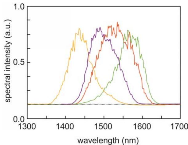
Figure 8: Infrared output spectrum and tunability of the White Dwarf IR OPCPA
