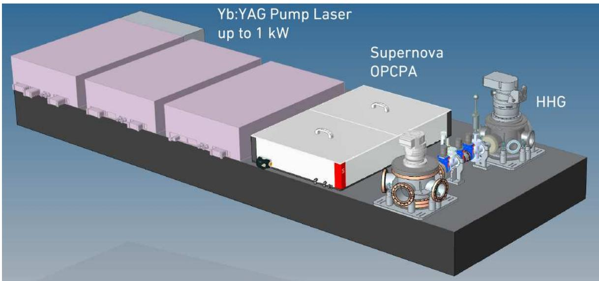
Figure 5. Schematic of a complete 100 W OPCPA system from *Class 5 Photonics GmbH*, with an optional HHG output.
