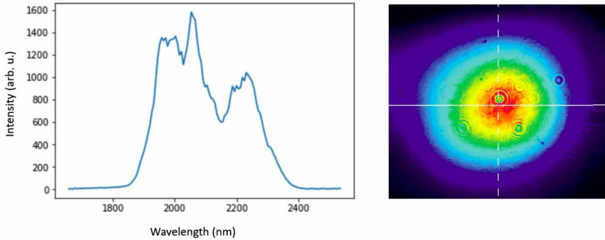
Figure 4. Typical OPCPA pre-amplified spectrum centered at  $2.1 \mu\text{m}$  (left). Gaussian beam profile of the amplified  $2.1 \mu\text{m}$  seed signal (right).
