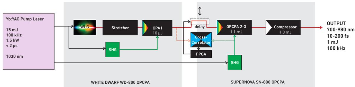
Figure 1. General schematic for a femtosecond, broadband or tunable 100 W NIR (700 – 980 nm) OPCPA with three amplification stages. The OPCPA has two components: a seed generation and pre-amplification stage (*White Dwarf WD-HE-800*) and a high power booster stage (*Supernova SN-800* from Class 5 Photonics). WLG – white-light-generation, SHG - second harmonic generation, OPA – optical parametric amplifier, FPGA – field-programmable gate array.
