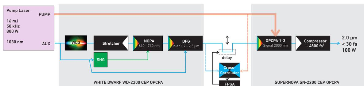
Figure 3. General schematic for a femtosecond, broadband, CEP-stable 100 W 2.1  $\mu\text{m}$  laser. The OPCPA has two components: a seed generation and pre-amplification (*White Dwarf WD-2200*) and a high power booster stage (*Supernova SN-2200* from Class 5 Photonics). WLG – white-light-generation, SHG - second harmonic generation, NOPA – noncollinear optical parametric amplifier and OPCPA – optical parametric chirped-pulse amplifier, FPGA – field-programmable gate array.
