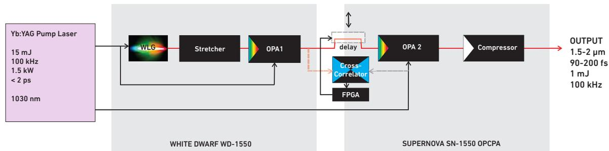
Figure 2. General schematic for a femtosecond, broadband or tunable 100 W SWIR (1.5 – 2.0 nm) OPCPA with a single booster stage. The OPCPA has two components: a seed generation and pre-amplification (*White Dwarf WD-HE-1550*) and a high power booster stage (*Supernova SN-1550* from Class 5 Photonics). WLG – white-light-generation, OPA – optical parametric amplifier, FPGA – field-programmable gate array.
