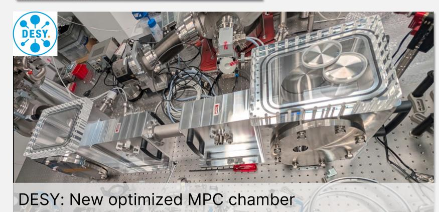
Target: > 600 W, 150 kHz, > 4 mJ Pulse duration: < 30 fs
